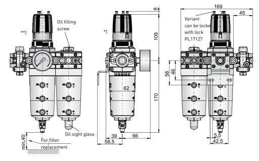
Air preparation unit, 2-piece with shut-off valve — model A15DVKL-1/2, -3/4
